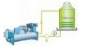
Water Cooled Chillers
